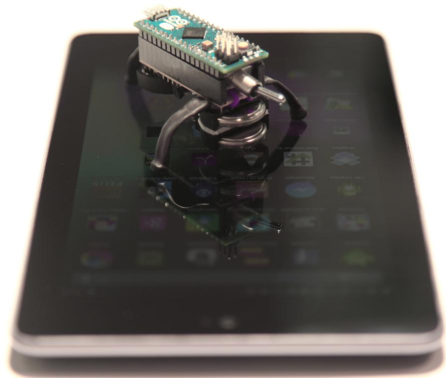
*Interfight is a physical, kinetic interface. It works by taking the human body capacitance as input, through conductive material, and interacts with another graphical interface on capacitive surfaces like touch-screens. The contact between both interfaces, cause a physical reaction (gravity, friction, vibration).*
